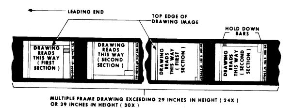
Fig 8-Multiple-Frame Drawing Section Image Orientation
