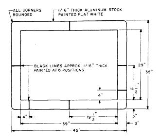
Fig 9—Guide for Microfilming Multiple-Frame Drawings at 24X Reduction
