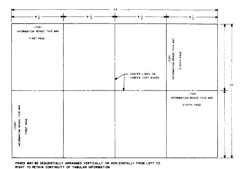
Fig 12-Layout for 8-1/2 by 11-Inch Pages (30X Reduction Format)
