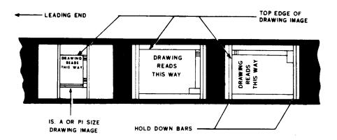
Fig 14—Single-Frame Drawing Image Orientation
