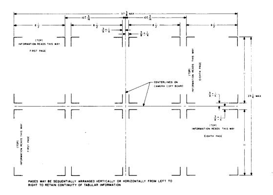
Fig 11-Layout for 8-1/2 by 11-Inch pages (24X Reduction Format)
